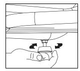
3. When the EFX is level, fully tighten the lock nut and lower the EFX to the floor.
