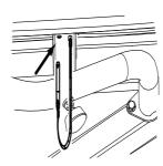
Figure 3: Store the locking pin under the ramp
